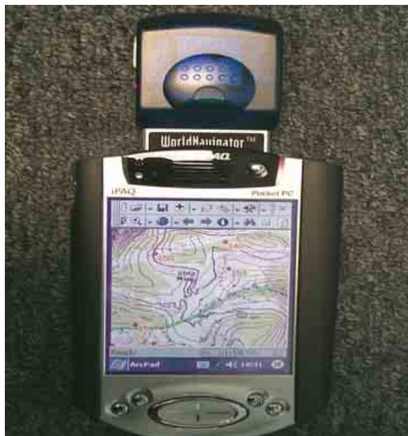
Figure 2. Moving map capabilities, which combine GPS and GIS technologies, can significantly reduce the time required for field investigations
