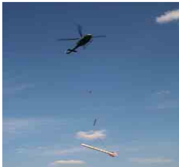
Figure 1. Helicopter with sling load of geophysical instruments
